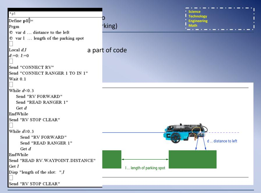
From the first steps with Rover to autonomous driving (parallel parking)
