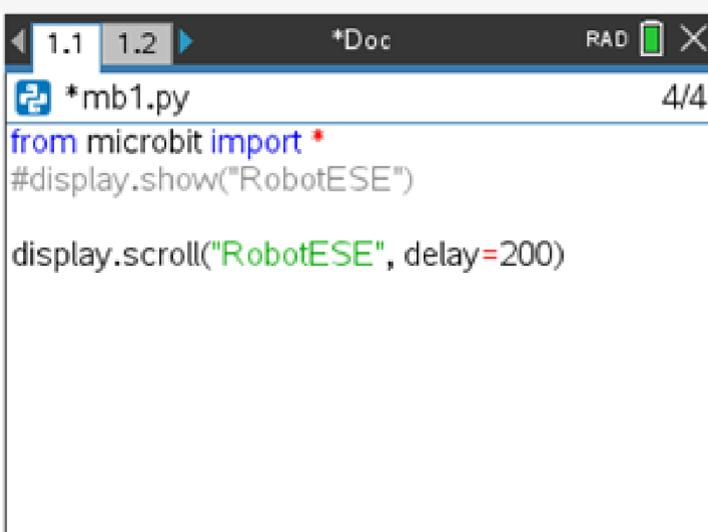
The speed at which the expression is moved can be controlled by adding the "**delay=**" parameter
